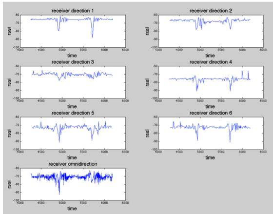
**Figure 6: RSS variance comparison between the directional antenna and omni-directional antenna**
