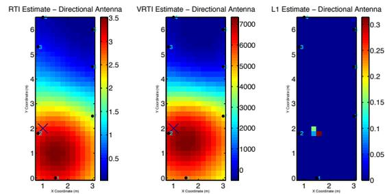
**Figure 7: Localization results using mean-based RTI, variance-based RTI and L1 RTI**
