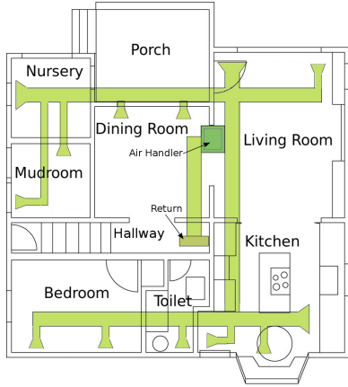
Figure 9. For realistic energy calculations and predictions, we created and empirically validated an energy model of the house and HVAC system shown here.
